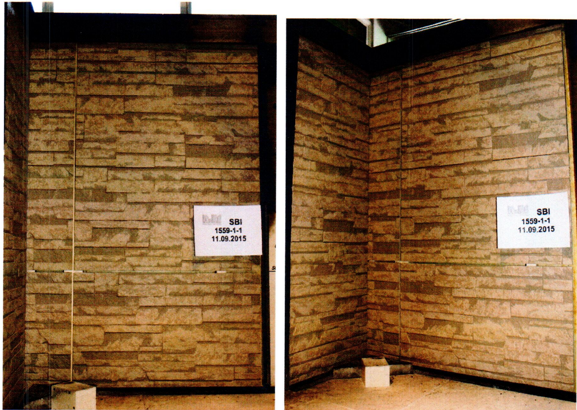
Fig. 1 Specimen mounting in SBI.
